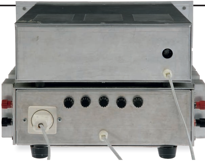
ABOVE: While the power amplifier rear panel carries an array of fuses, the preamplifier input/output phono connections are neatly arranged to one side
